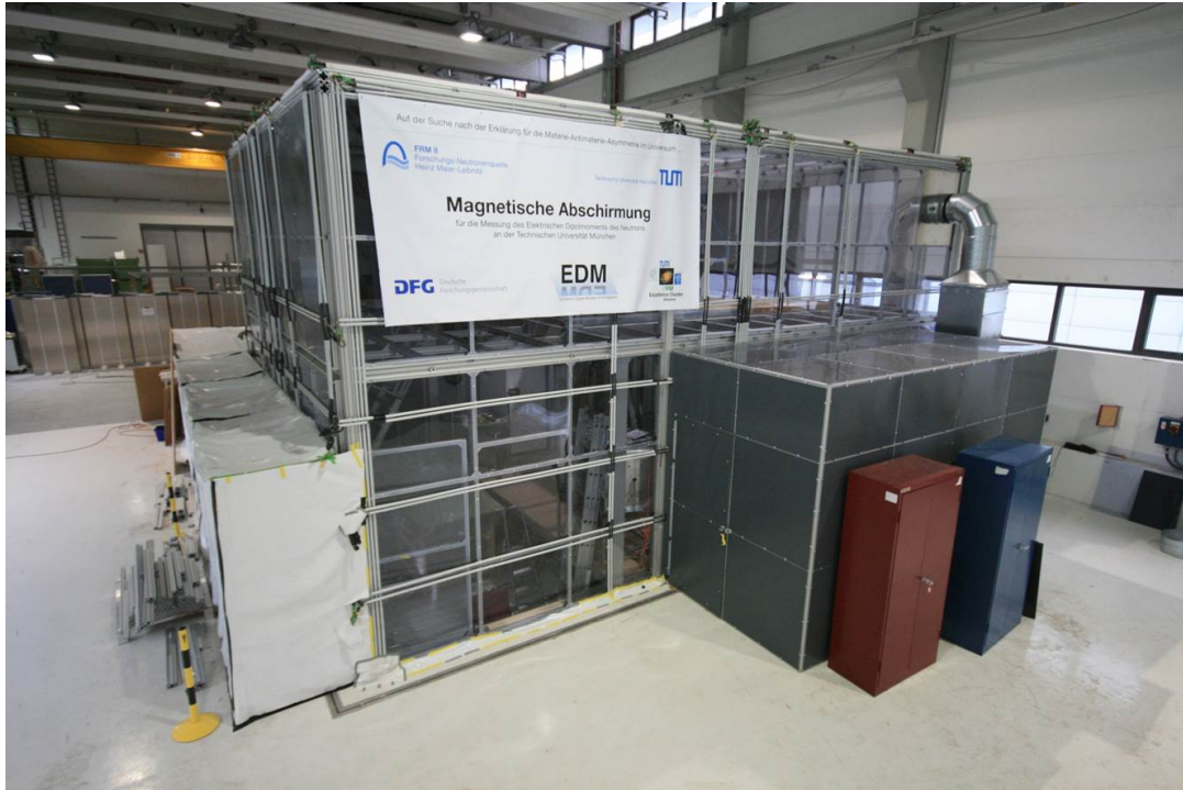
Figure 3.3.: Photograph of the field cage after its construction: An aluminum structure supports the hull made of PVC panels and the cables of the coils (kept in place with PVC tubes).
