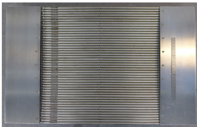
Figure 1: Detector segment with 48 detector tubes in a curved assembly.
