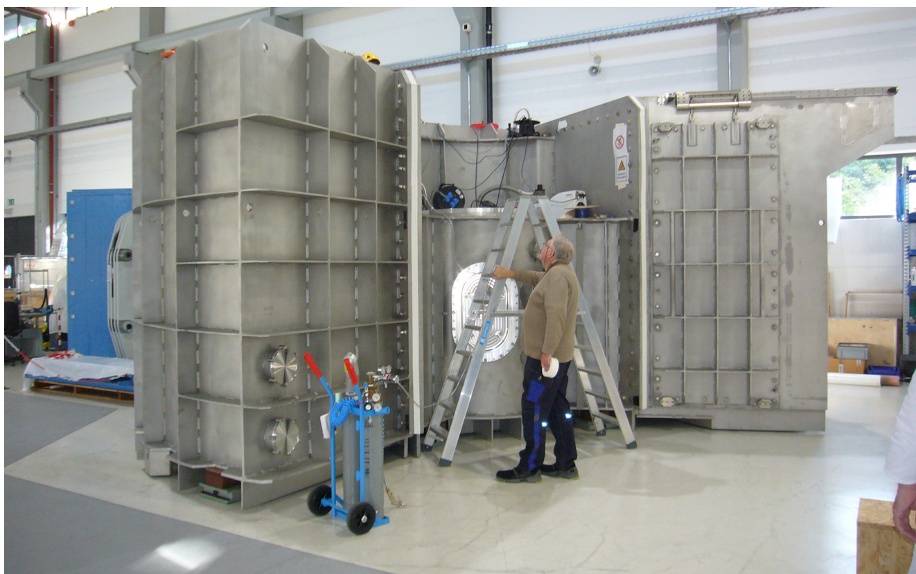
Figure 3: TOPAS high vacuum chamber in the guide hall east during leak testing.
