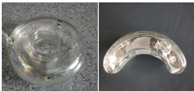
Figure 17: Left, a photo of a doughnut shaped cell “Homer” for PASTIS testing made of GE180 produced in FZ-Jülich by P. Pistel (glassworkshop ZEA-1 FZ Jülich) which has 0.5 bar ^3\text{He} gas and a 1074 hour relaxation time. Right, a C-shaped cell that has uniform path length for wide-angle neutron scattering experiments, the “Marge” cell has a 120^\circ coverage and a 160 hour relaxation time with a fill pressure of 1.1 bar of ^3\text{He} gas.
