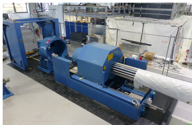
Figure 19: Setup for cold tests of the replacement of plug JMA05.
