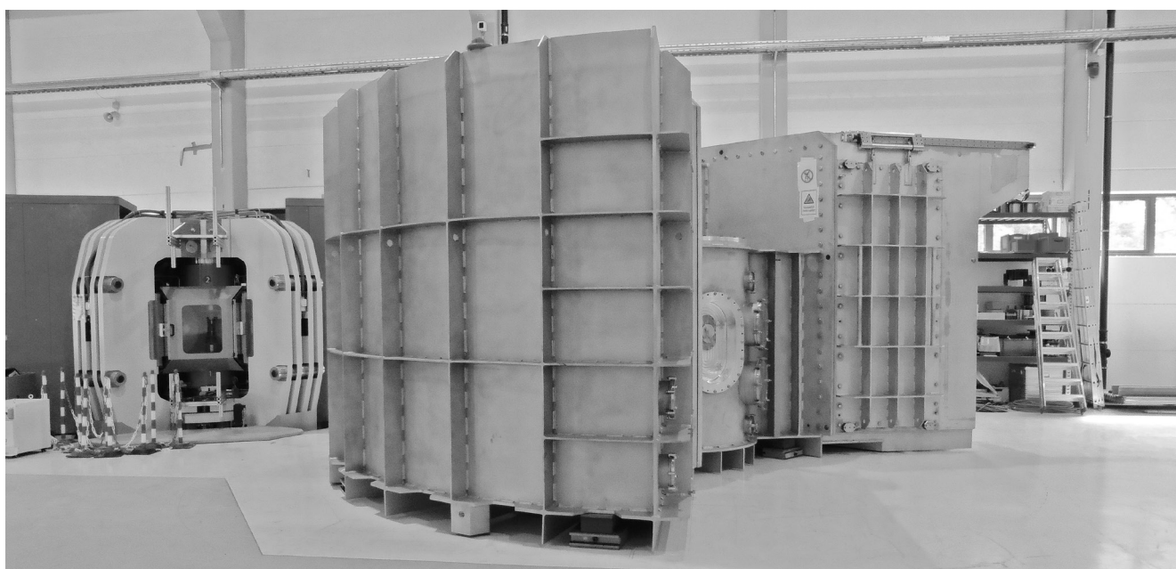
Figure 19: The assembled TOPAS spectrometer chamber in the neutron guide hall east.
