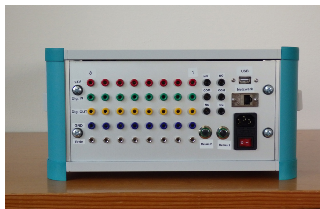
Figure 4: Plug'n Play digital I/O box to be used easily with TACO and NICOS instrument control software.
