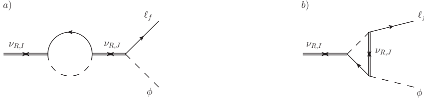
Figure 2.3: One-loop self-energy and vertex diagrams that interfere with the tree level diagrams for the decay process \nu_{R,1} \rightarrow \ell_f + \phi . The notation of the particles is the same as given in figure 2.2. The neutrino propagators with forward-backward arrows correspond to \langle 0|T(\psi\psi)|0\rangle or \langle 0|T(\bar{\psi}\bar{\psi})|0\rangle . Similar diagrams exist for the decay process \nu_{R,1} \rightarrow \bar{\ell}_f + \phi^\dagger .
