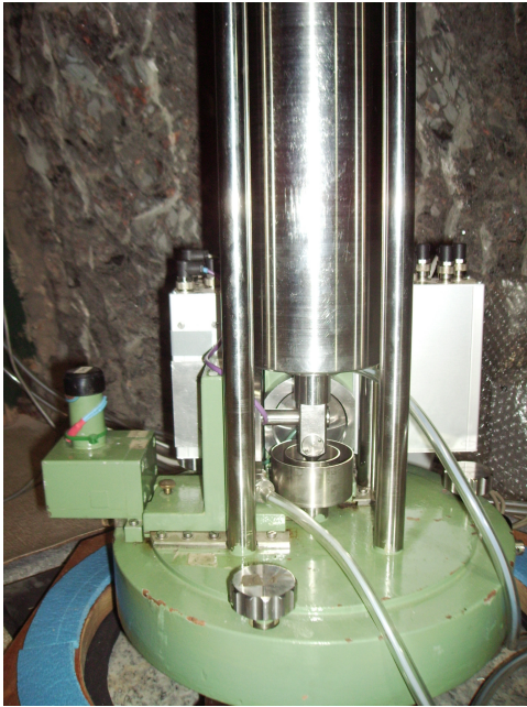
Fig. 3.11: Measurement unit with pendulum mass before update.
