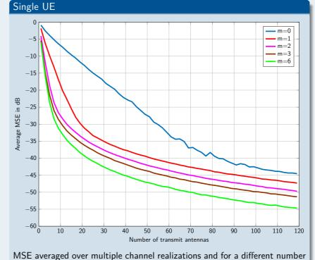
MSE averaged over multiple channel realizations and for a different number of bits for the phase information (m) with the Rayleigh channel model
