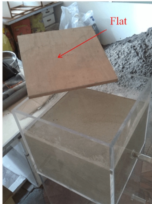
Figure 4.2 Soil filling into the tank model. Every 5cm depth soil layer is pressed by the flat uniformly.
