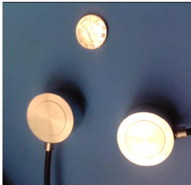
Figure 4.5 Pore water pressure transducers
