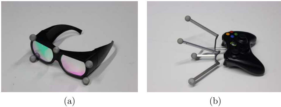
Figure 3.3: (a) A pair of shutter glasses with markers attached for tracking the user. (b) An Xbox 360 controller attached with markers to control the scene.
