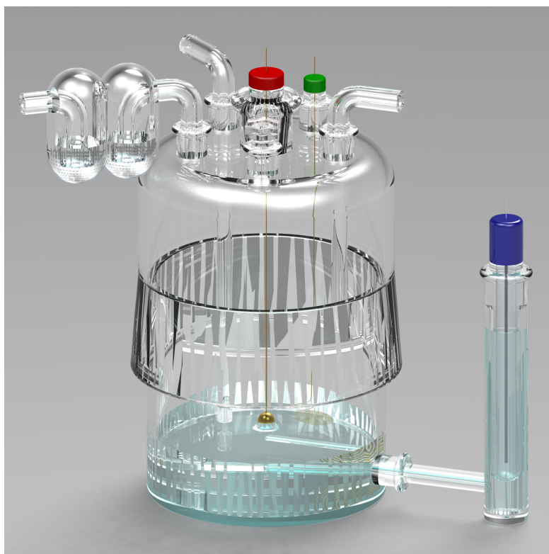
Figure 3.1.: Model of an electrochemical glass half cell. The main compartment (left) contains WE (red), CE (green), two gas inlets and a gas outlet. The RE (blue) is connected to the main compartment via a Haber-Luggin capillary.
