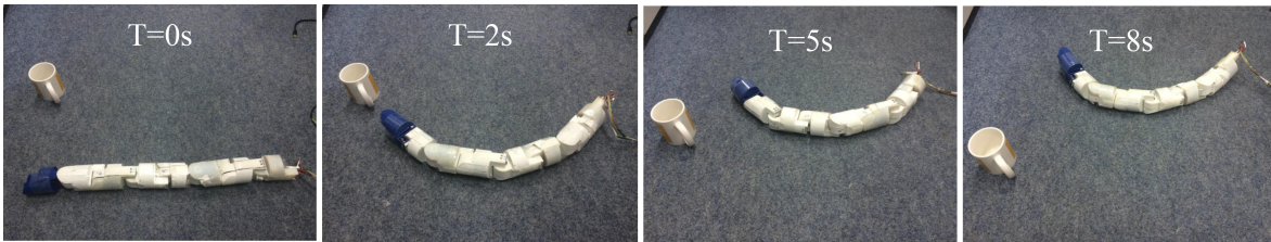
Fig. 14. Snapshots of the robot rolling, the CPG parameters: amplitude 30^\circ , frequency 0.2Hz, phase differences are set as Equation.17.
