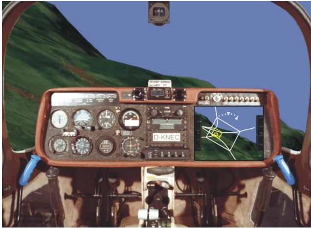
Fig. 9 Cockpit instrumentation with predictor-tunnel display (banked flight condition)
