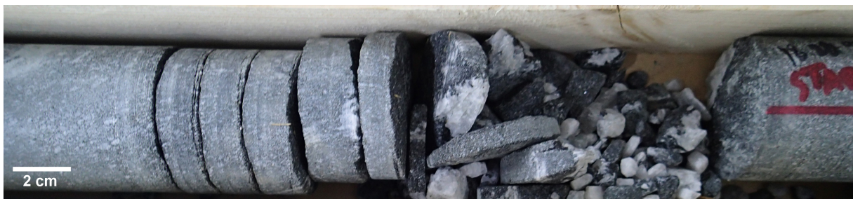
Figure 51: Core diskings observed in a section of the drilling with weaker core material where stress concentrations at the drill bit exceeded the crack initiation stress.
