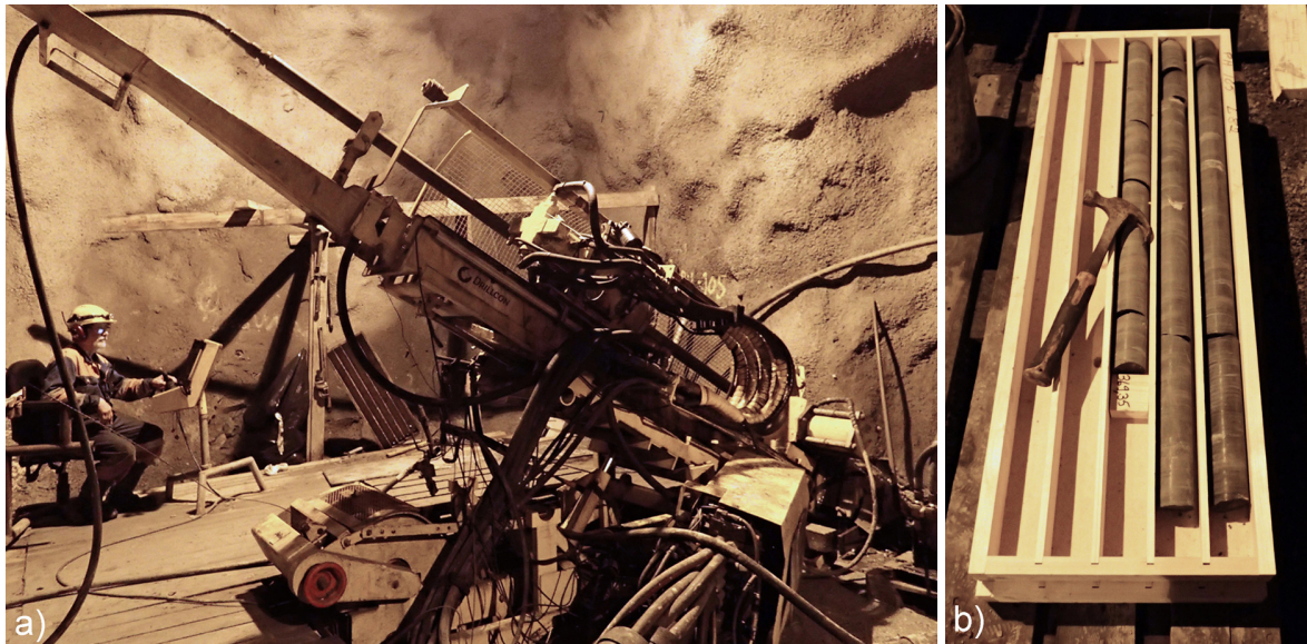
Figure 41: a) Drill rig at borehole PH105 at the level +1080 with an azimuth of 330^\circ and an inclination angle of 30^\circ . b) Samples of the mafic volcanic rock were selected from the drill core immediately after core recovery.
