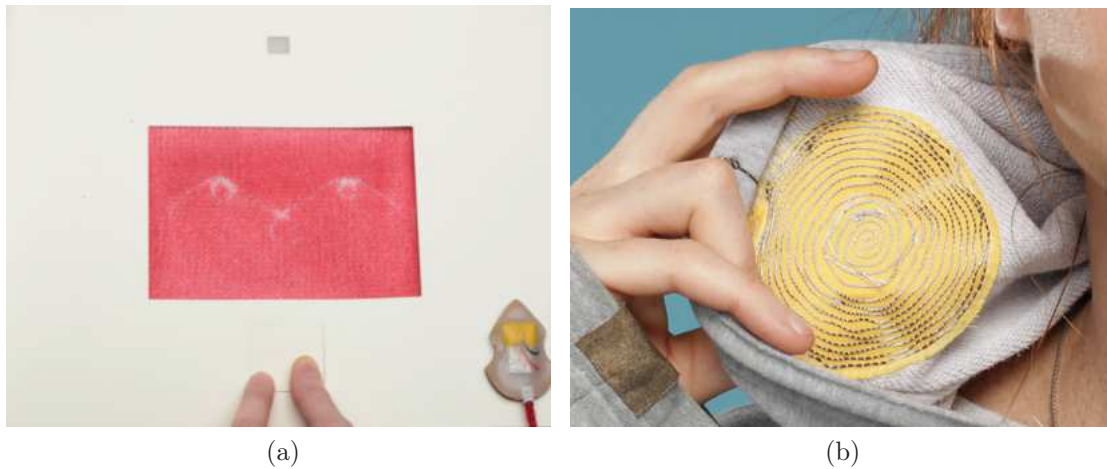
Figure 2.12: Textile output devices. a) Textile thermochromic display. Reprinted with permission of Katharina Bredies. b) Textile thermochromic display. Reprinted with permission of Katharina Bredies.
