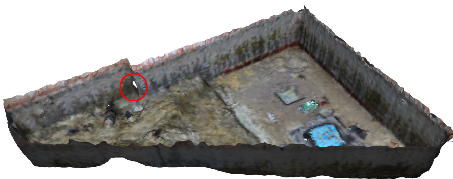
Figure 6.14: Meshed surface of the point cloud in Figure 6.10. The surface was generated using the ball pivoting algorithm by Bernardini et al. (1999). The red circle shows a hole that was left open.
