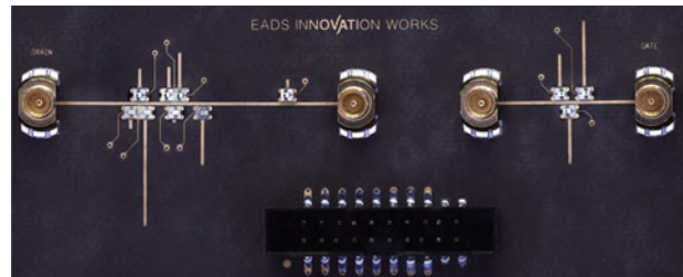
Fig. 7. Top view of assembled M 3 N. Left structure: output matching network, right structure: input matching network. Left port of structures: transistor side, right port: 50 \Omega system. "GATE" is accidentally placed on the wrong side of the structure. Reference planes 8 mm inwards from center of RF connectors.
