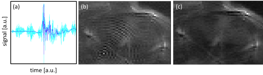
Figure 7.1: De-noising of multi-spectral OA data. (a) Signals of one projection at 900 nm laser wavelength before (cyan) and after (blue) de-noising. (b) Corresponding original, noisy reconstruction. (c) Corresponding reconstruction from the de-noised signals with improved image quality.
