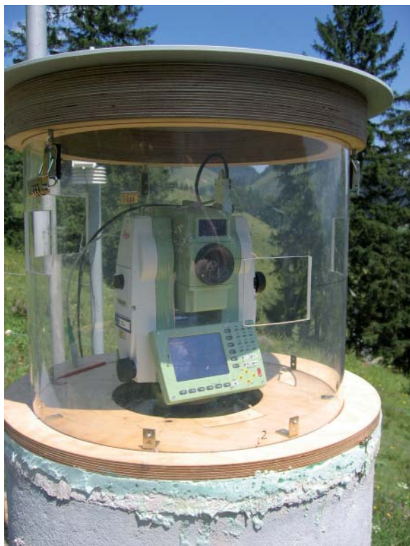
Figure 11: VTPS prototype in its housing at the Aggenalm Landslide test site (Singer et al. 2009a).
