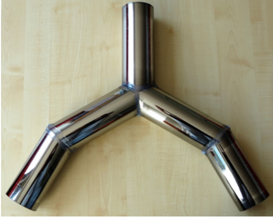
(a) Beam splitter No. 1 (BS No.1) with an opening angle of 120^\circ with a 30^\circ chicane for the simultaneous spin detection part
