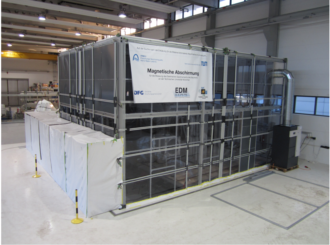
Figure 2.5: Picture of the magnetic shield with the active compensation system around. According to Fig. 2.4
