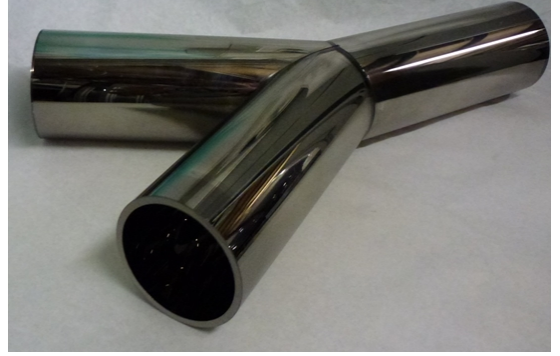
(b) Beam splitter No. 2 (BS No.2) with an opening angle of 60^\circ between the dividing legs of the beam splitter
