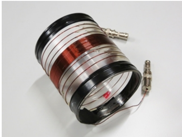
Figure 5.3: Picture of a broadband adiabatic spin flipper for the future nEDM setup with an inner diameter of 100 mm and a length of 110 mm with 30 windings of a 1 mm copper wire.
