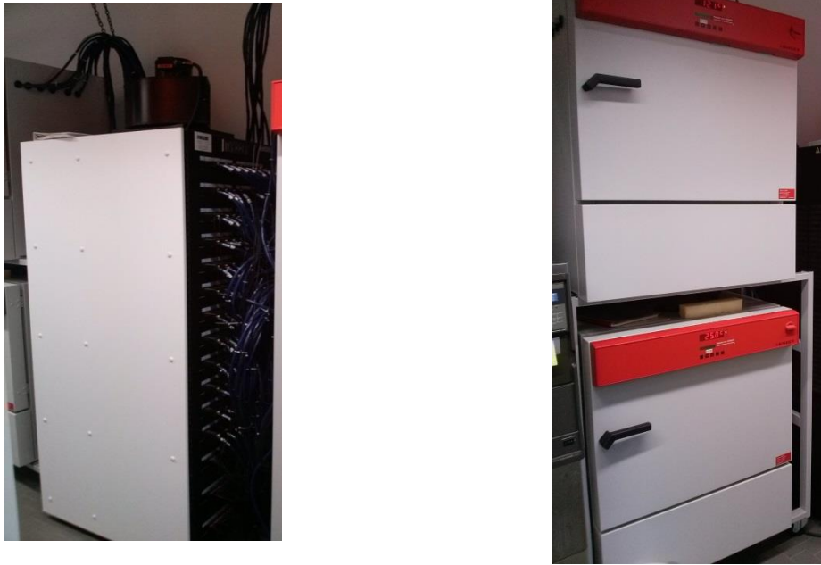
Figure 23: Battery test cycler with 64 channels and climatic chambers for a constant temperature during galvanostatic cycling
