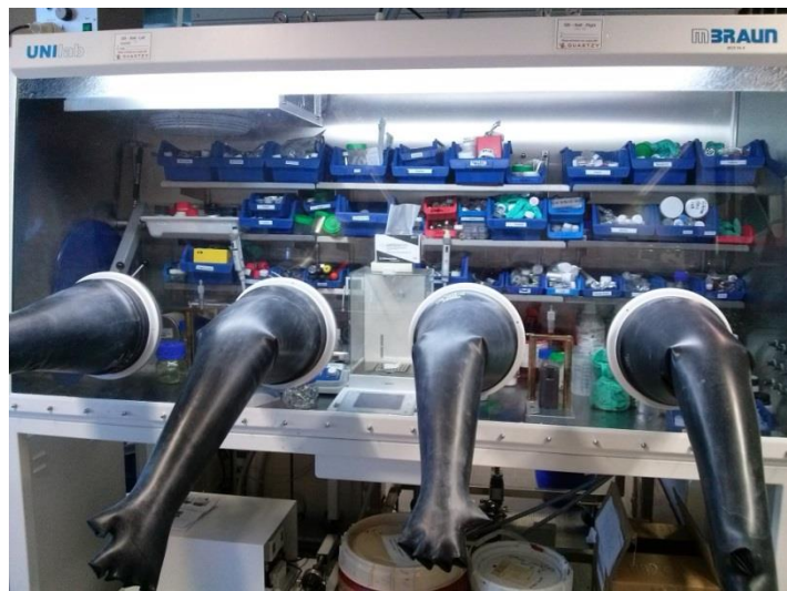
Figure 17: Ar-filled glovebox with semi-microbalance for weighing electrodes and for manufacturing battery test cells
