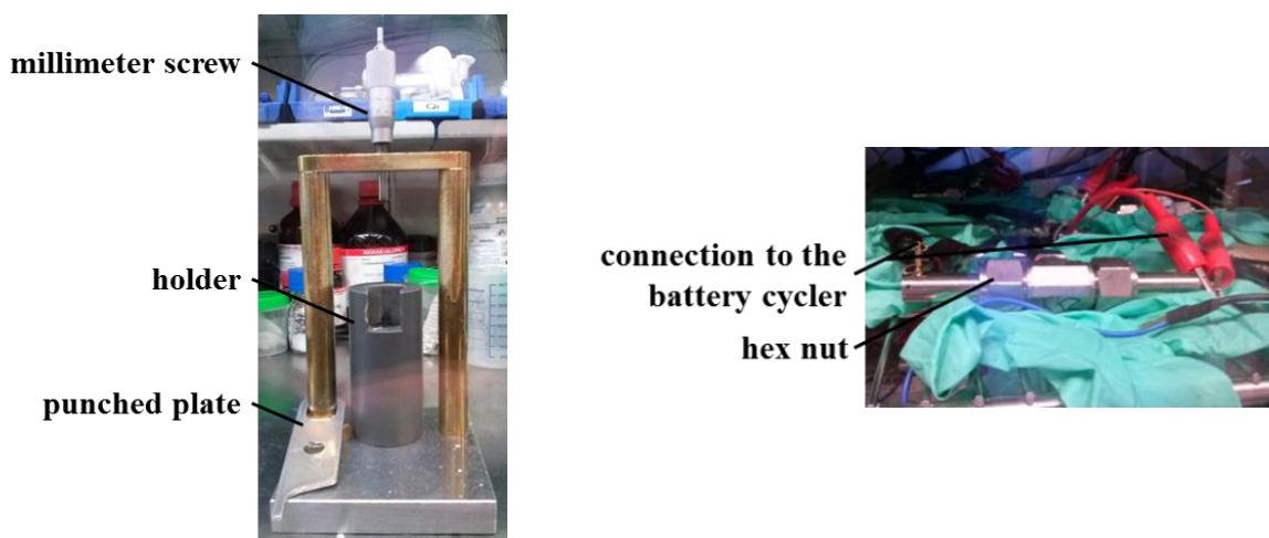
Figure 22: Costum made tool for battery test cell assembly and finished test cell connected to the battery cyclor (MACCOR)
