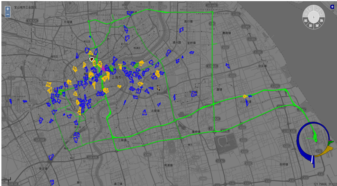
Figure 8: User interface showing the drop-off clusters and their functions: - public building (blue), commercial buildings (yellow), residential building (green) and industrial building (magenta); Trajectories between Pudong airport and destinations (green lines of varying density) (Ding et al. 2015b)
