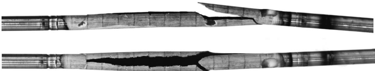
Figure 5: PCMI failure mode observed in the NSRR test VA-1 (PWR, 71 MWd/kgU, cladding ZIRLO™) [47]
