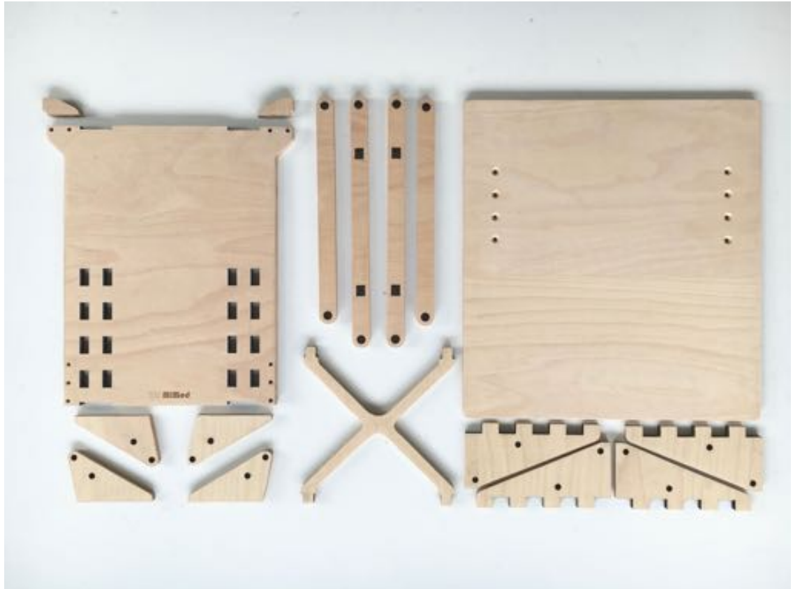
Figure 45 Manufactured wooden components of the modular lift-assist chair
