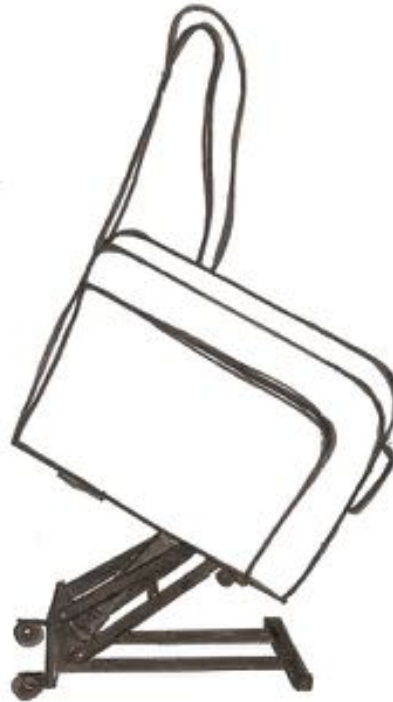
Figure 10 Conceptual design of a stand assist lift based on (Curdija et al., 2010) (Drawing by Kyra Kleine)
