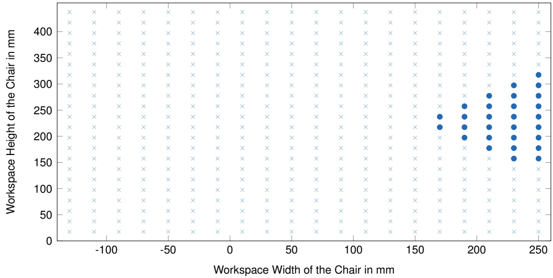
Figure 51 5th male percentile results of an exhaustive search for positions of moving pivot points within the rectangular workspace of the chair
