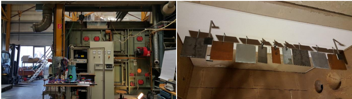
Figure 4: Furnace (left) & test specimen with different surfaces (right)
