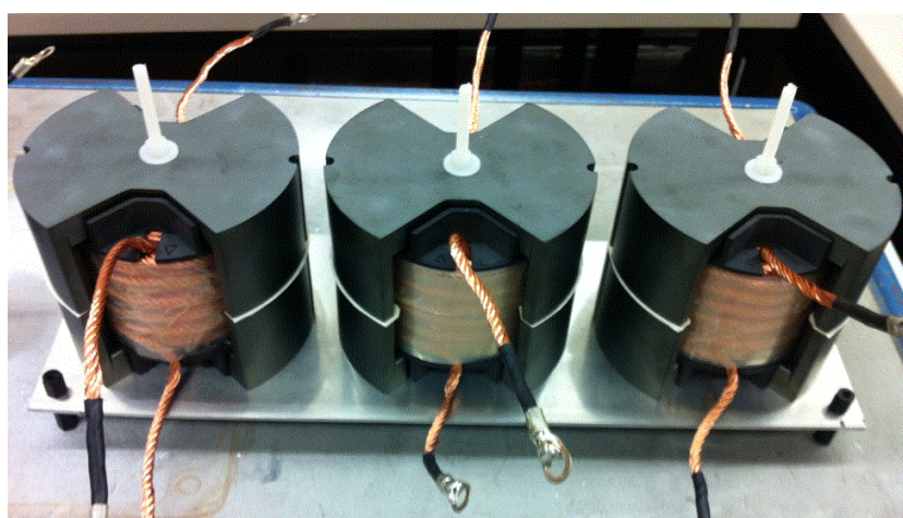
(c) Final three phase coupling inductor.
