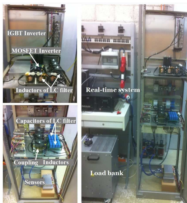
Figure 6.2: Experimental setup of the prototype grid emulator. Upper left: power stage and inductor. Bottom left: coupling inductors and capacitors. Right: Overview of the system.
