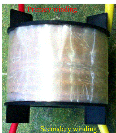
(a) Picture of the coupling inductor winding on the bobbin.
