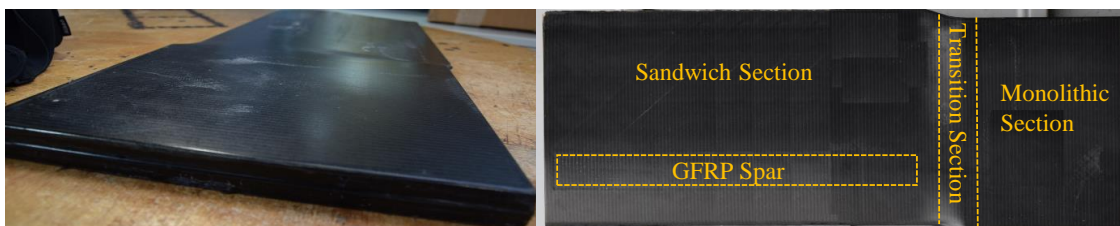
Figure 7-1 Different material sections of the generic rotor blade.
