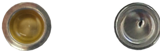
Figure 3-2 Weight loss specimen without lid (left) and with lid (right). The right specimen is similar to the specimens measured in the DSC.
