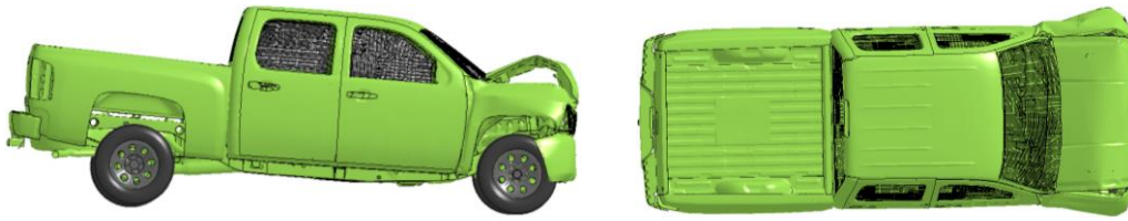
Figure F.7: Deformations of Chevrolet Silverado against the FWRB at 50 km/h after 200 ms
