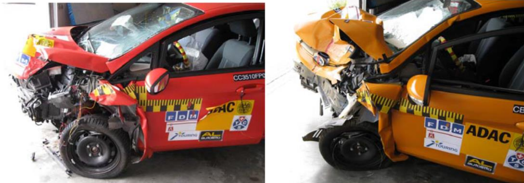
Figure 4.19: Deformations in car-to-car test (left) and car-to-MPDB test (right) [14, p. 9]
