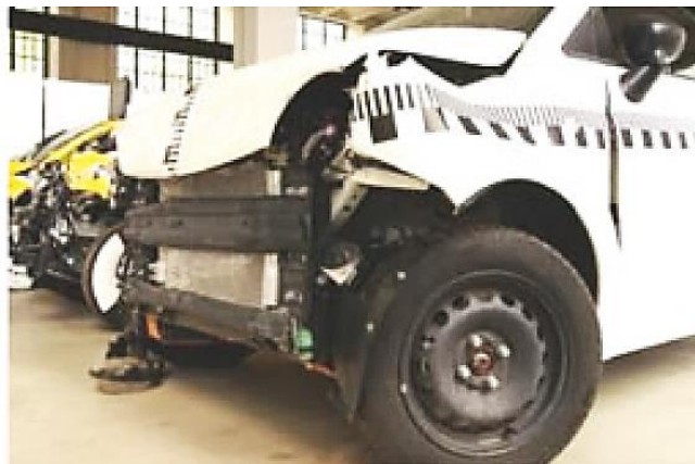
Figure 4.1: Unrealistic deformation pattern in the FWRB test [98, p. 111]
