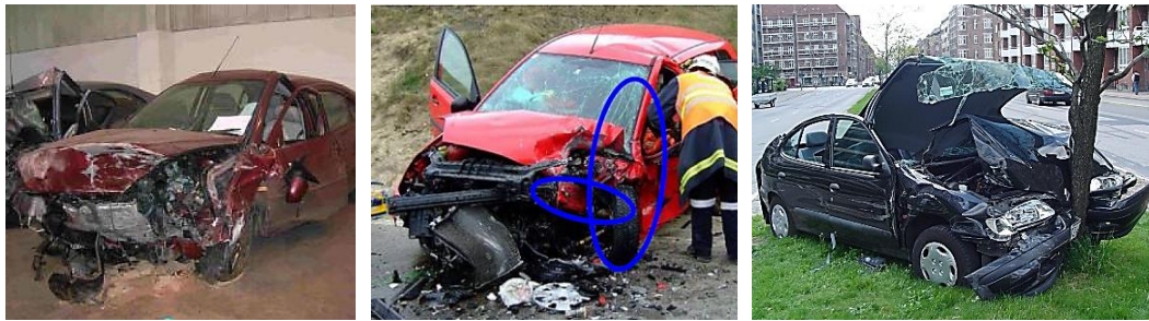
Figure 2.16: Samples of geometry incompatibilities; Over/underride (left), small overlap (middle), and the fork effect (right) [91, p. 53]; [14, p. 2]; [96]
