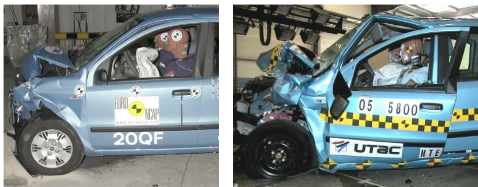
Figure 2.17: Deformations of a supermini in the ODB test with a 40 % offset at 64 km/h (left); in an equivalent car-to-car collision with a mass ratio of 1:1.3 (right) [97, c11-c12]
