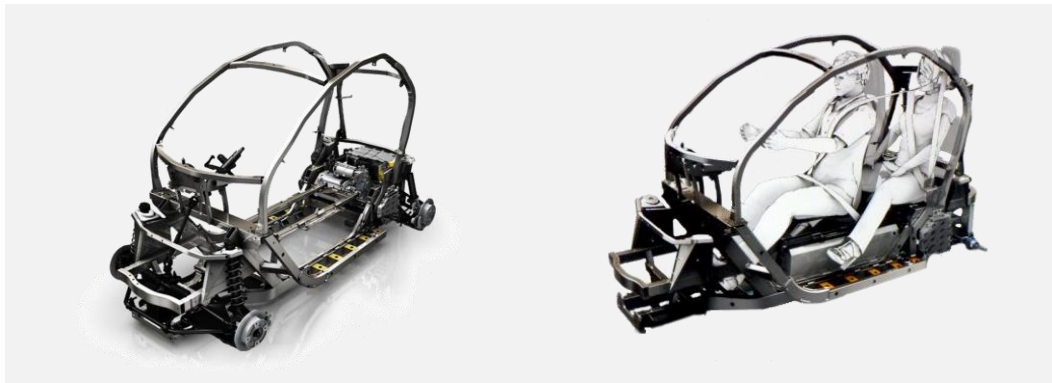
Figure 2.12: Vehicle structure and occupant compartment of the Renault Twizy [80], [81]
