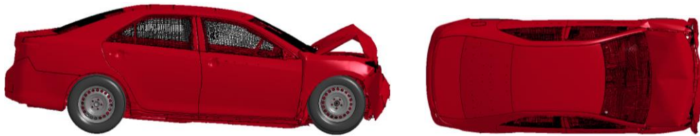
Figure F.5: Deformations of Toyota Camry against the FWRB at 50 km/h after 200 ms
