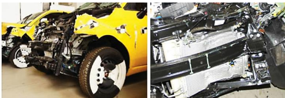
Figure 4.2: Comparison of front structure deformation pattern in different frontal impact tests: FWDB test (left), car-to-car test (right)
