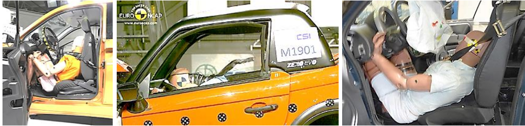
Figure 2.11: Ligier IXO (left), Tazzari Zero (middle), and Microcar M.Go (right) in frontal impact test of Euro NCAP
