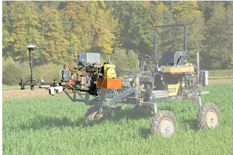
Figure 3.8.: Phenotyping platform PhenoTrac 4 of the Chair of Plant Nutrition from the Technical University of Munich
