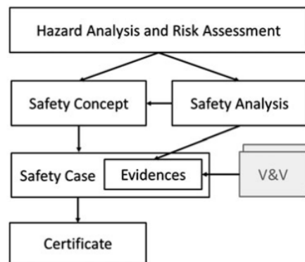
Figure 2.7: Safety engineering lifecycle from [336]
