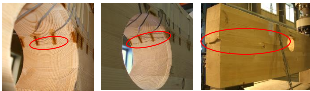
Figure 3: Stepwise failure characteristics (left: crack initiation; middle: full crack; right: ultimate load)
