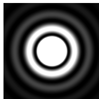
Figure 3.1: Airy disk pattern produced by light passing a circular aperture. The gray level scale has been adjusted to the maximum of the first ring, to make the outer rings visible.
