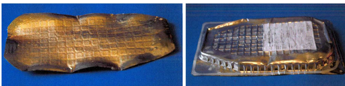
Figure 6-3 Left: Cardboard inlay after HPP. Right: Example of an unsuitable packaging design. Own unpublished results from investigations made for industrial clients.
