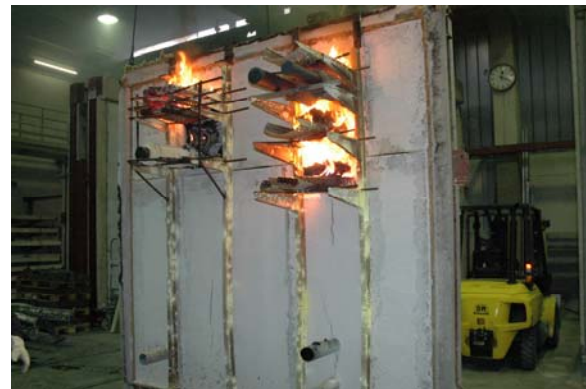
Figure 6: full scale fire tests of wall assembly with multi penetration sealing systems after fire test (picture DGFH)
