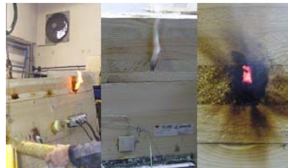
Figure 14: flame spread caused by gaps in CLT elements
