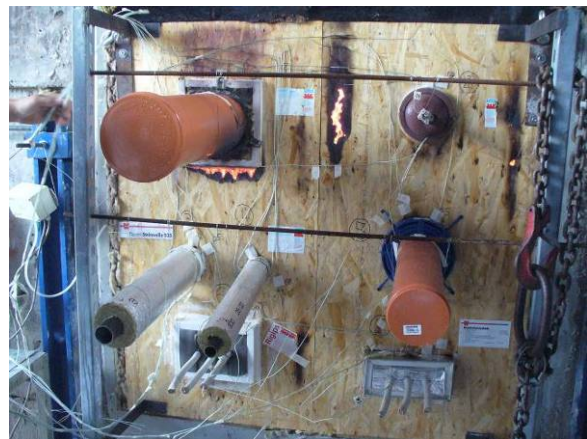
Figure 9: failure of small scale timber frame assembly (EI 30) after 43 minutes
