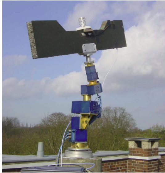
Figure 13.1 GOCE GPS antenna set-up for near-field multipath calibration using a GOCE mock-up as originally proposed to ESA (GOCE Project Office) in (Švehla and Rothacher 2004d). (credit ESA)
