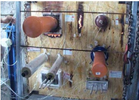
Figure 6. Failure of small scale timber frame assembly
