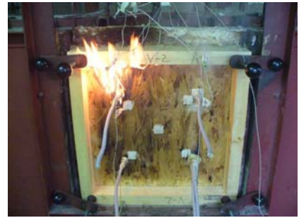
Figure 3. Failure at penetration sealing with non fire retardant PU foam
