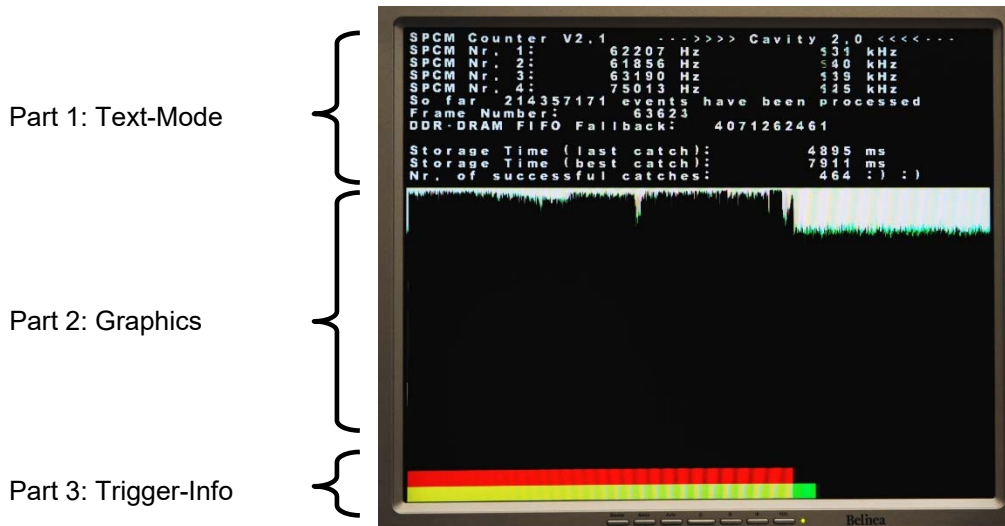
Figure 10.10: Displayed output of the VGA interface. The output is divided into a text, a graphics and a triggering part.
