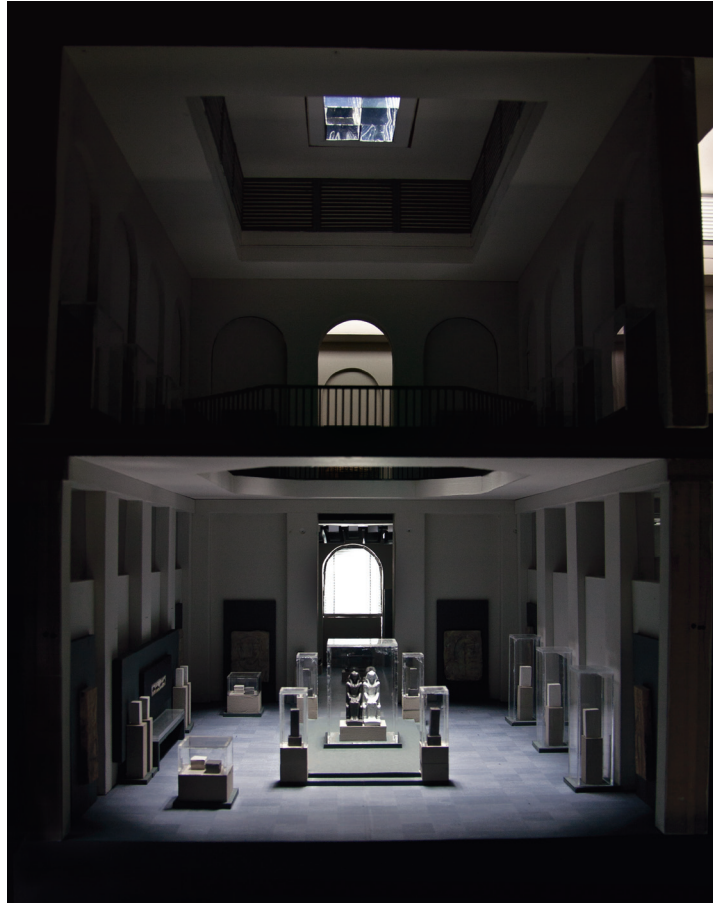
Figure 5.138 The light atmosphere in the Large Side Hall GF. The chamber system directs the light to the entire ground floor area. It creates a smooth light distribution from the centre of the space to the wall, that highlight the platform and the masterpiece. The reflected light from the floor illuminate the walls and the ceiling with a dim, soft light. The systems is glare free from both floors.
