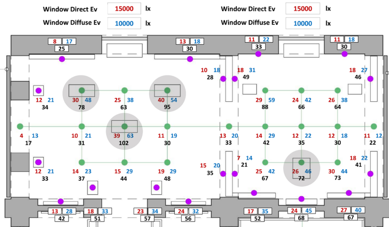
Figure 5.164 The daylight illuminance values in the Lateral Gallery GF in the afternoon on 21 Mar at 13:00 when 25 klx external daylight illuminance is measured to the normal of the windows. A fish system with a roller-screen is installed in the windows and a reflective ceiling in every zone.
