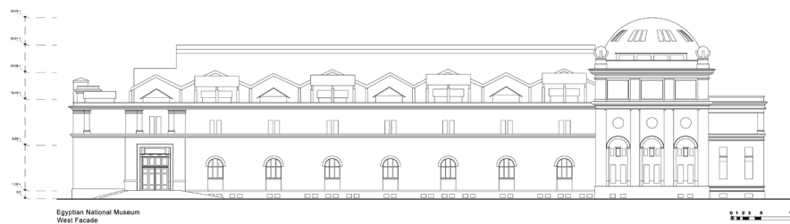
Figure 5.33 The west facade. Note: the existed concrete protection roof is added to this drawing and absent from the previous section drawings. (after modifying the drawings by Shaker Consultancy Group in 1999).
