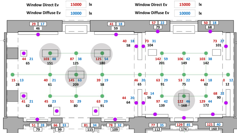
Figure 5.166 The daylight illuminance values in the Lateral Gallery GF in the afternoon on 21 Mar at 17:00 when 25 klx external daylight illuminance is measured to the normal of the windows. A fish system with a roller-screen is installed in the windows and a reflective ceiling in every zone.
