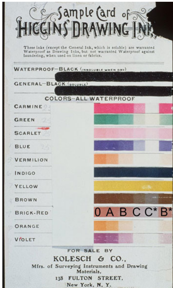
Figure 3.10 Drawing inks on paper faded by daylight through glass. (Canadian Conservation Institute, www.cci-icc.gc.ca ).
