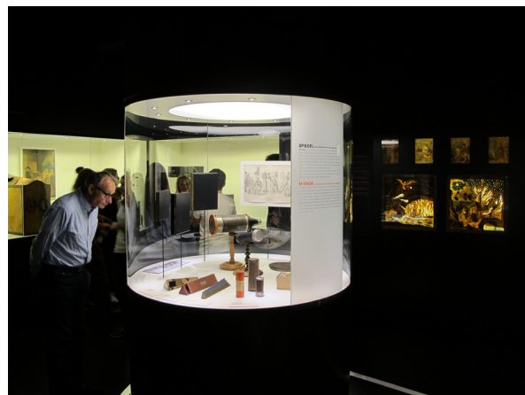
Figure 1.90 Showcase with white interior and it is internally illuminated with LEDs and a small diffuser-ceiling. The gallery interior is black and the general illumination depends on the stray light from showcases. (The German Film Museum, Frankfurt, Germany).
