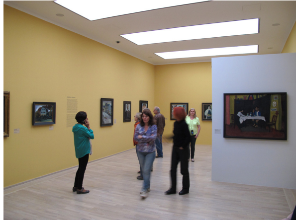
Figure 1.58 Reducing the size of the luminance ceiling in small galleries give more control on glare and light distributions. (New modern wing of the Lenbachhaus, Munich, Germany).
