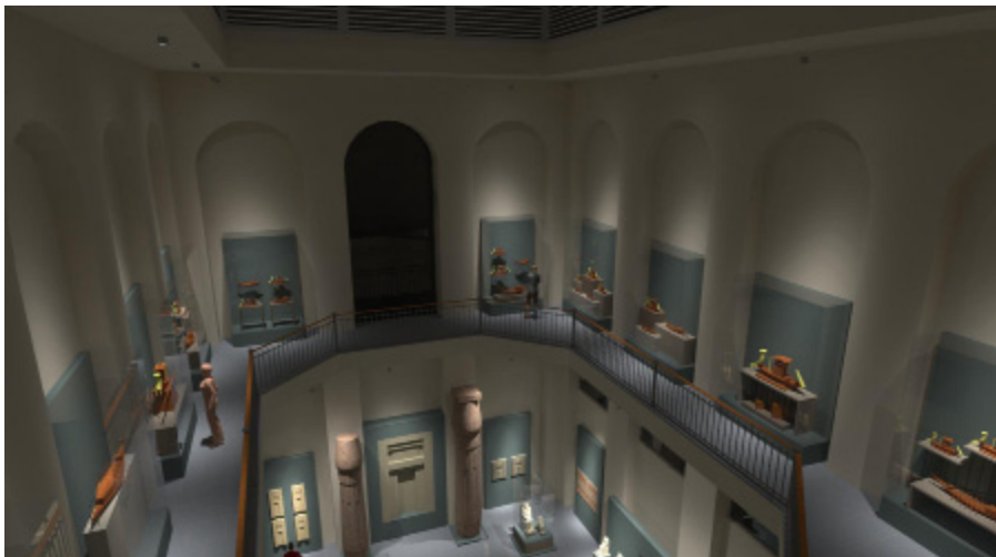
Figure 5.195 The dramatic atmosphere in the Large Side Hall GF. There is enough lights in front of the showcases, however the walls and the ceiling is dark and visitors can not see the architecture of the gallery.
