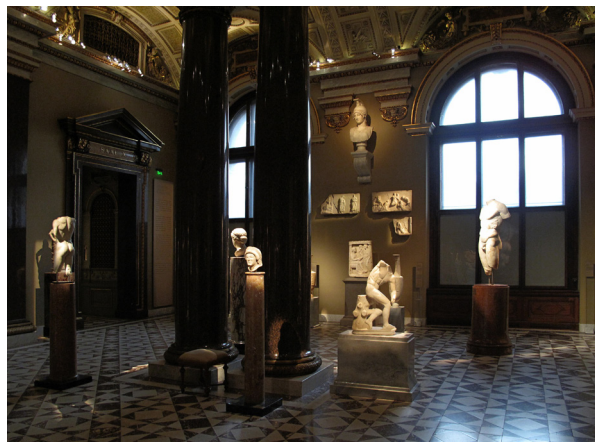
Figure 1.69 Classical Greece statues illuminated with projectors mounted over the wall cornice. The room lighting is the daylight from the windows' diffuser panel. (Museum of Art History, Vienna, Austria).
