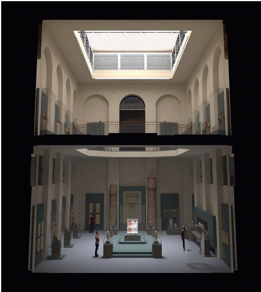
Figure 5.181 A ray tracing rendering shows the room lighting distribution created with the artificial light in the Large Side Hall GF & UF. The ray tracing rendering are generated by Relux software. (Compare with Figure 5.140)
