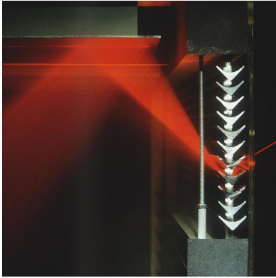
Directed transmission as a function of angle of incidence beam light
