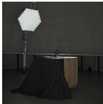
Figure 5.105 (left) Second system in comparison: a horizontal diffuse glass panel closing the CPC opening.
