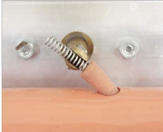
Figure 7. The papilla is inserted into the opening of duodenum and fixed to the mount by gently pressing its metal coil into the groove of the mount. The metal coil serves for grounding the papilla via the mount connected to a socket at the back. When the carriage is closed, the coil leads instruments inserted into the papilla into the bile duct. This can be viewed in the window of the simulator.
