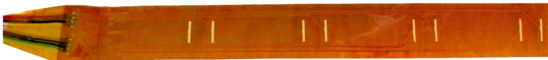
Figure 7.4 The sensor strip array used for the measurement. The four sensor spots are placed every 5 cm. The distance between the electrodes of one sensor spot is 1 cm.
