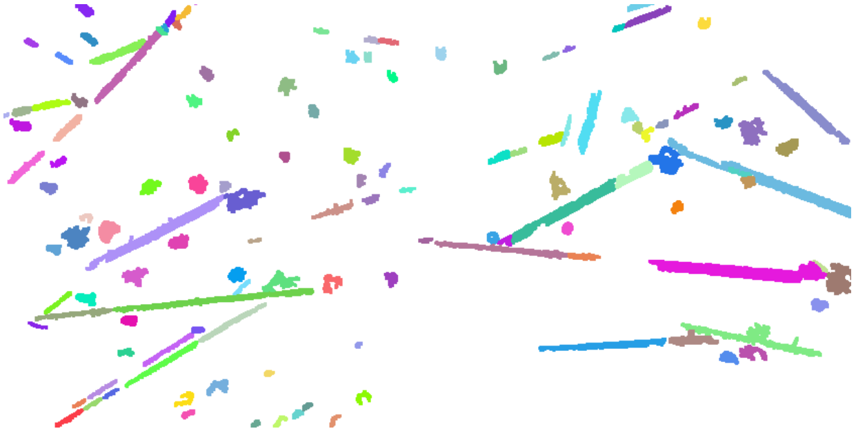
Figure 4.12: Connected components of high-probability stem points (random colors). Elongated structures represent fallen trees, smaller clusters are parts of standing trunks.
