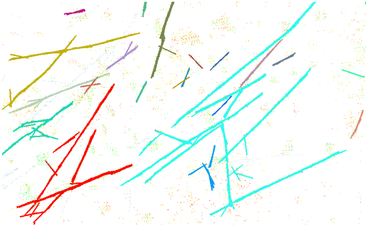
Figure 4.11: Set of segment candidates partitioned into disjoint networks, represented by different colors. Each network is independent of the others and can be processed separately.
