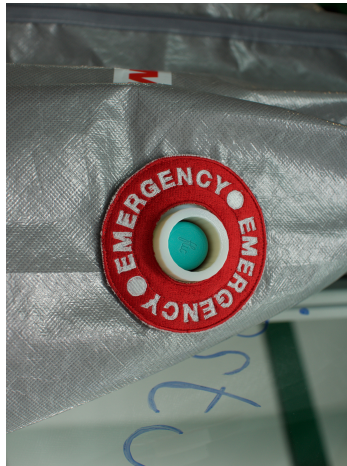
(b) Textile Interface: the Emergency Button consists of a stitched label that is attached with Velcro. A 3D printed button protection prevents accidental button pushes. For the prototype we used a Flic Button.
