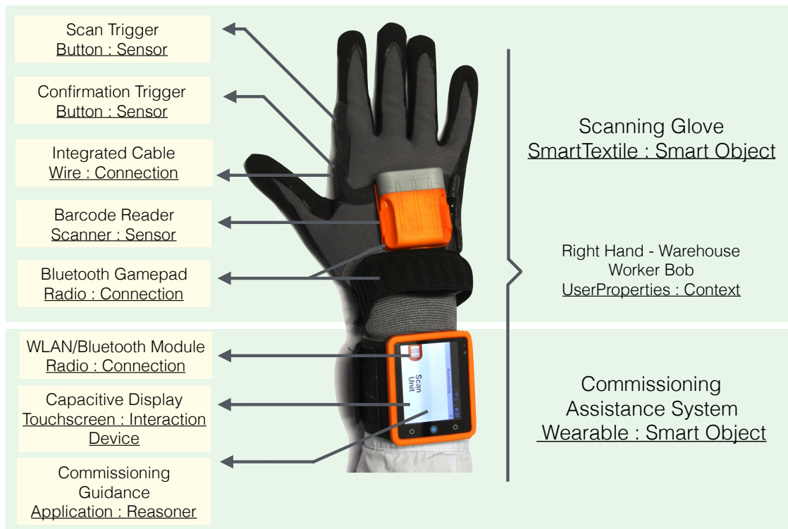
Figure 2.12: Top-Level Design of Scanning Glove and Commissioning Assistance System: the figure shows two Smart Object extensions for the Smart Logistics application. Both use abstractions of the base-metamodel. The Scanning Glove uses Sensors, Connections, whereas the Commissioning Assistance System uses a Connection, an Interaction Device and a Reasoner.
