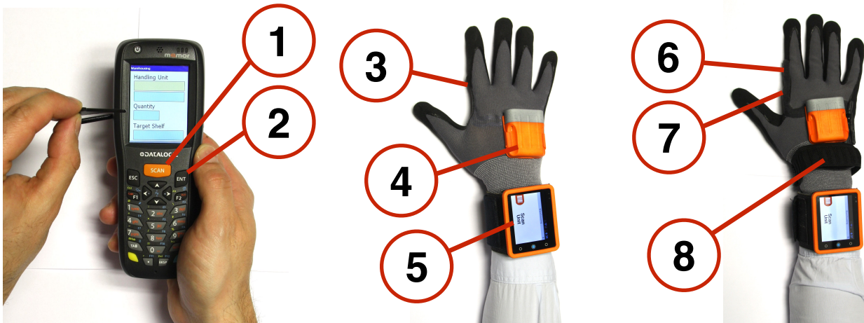
Fig. 1: Prototype Variants: The figure shows our three variants (from left to right): the handheld scanner, the smart glove with one button and smartwatch, and the smart glove with two buttons. The variants simulate a 'hands occupied' scenario (handheld scanner), a 'semi hands-free' scenario (one button) and a 'hands-free' scenario (two buttons). The annotated numbers mark the features of each variant as described in the text.
