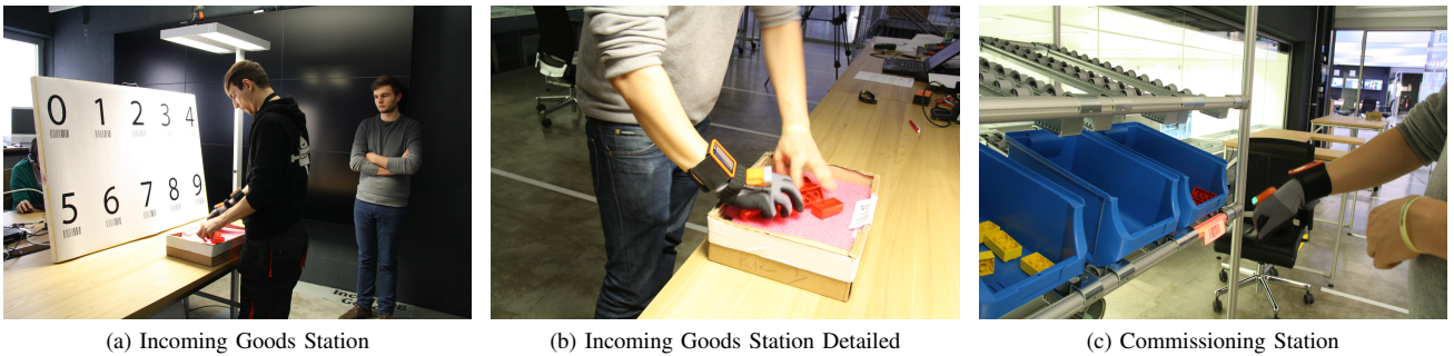
Fig. 3: Setup of the User Study: The pictures show our shop floor hardware setup. Picture 3a shows the 'Incoming Goods Station'. It shows the setup for the two buttons variant with the offered digit scan panel. The detailed view in picture 3b of the 'Incoming Goods Station' shows the package and the units (8 duplo® stones). The last picture 3c shows the 'Commissioning Station' with the attached barcode on the target shelf.
