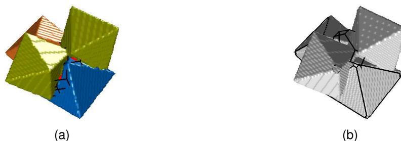
Figure 4.10: Segmentation (left) and shape identification (right) for one aggregate from sample A1-0. Two green primary particles were wrongly concatenated. The aggregate is considered to have an unsuccessful shape identification by both sets of quality measures.
