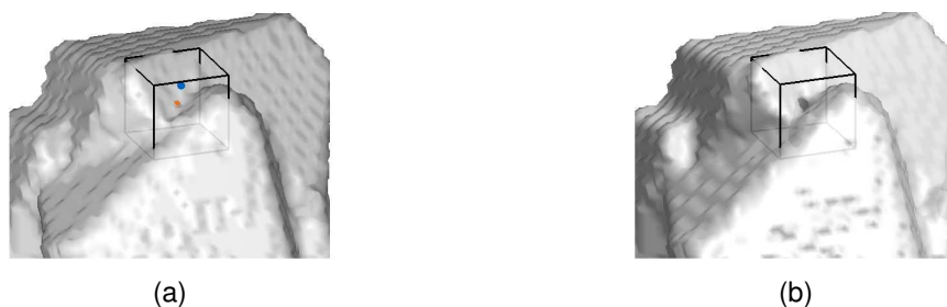
Figure 4.4: (a) Concavity expansion procedure deletes foreground voxels in the concavity direction, defined between the concavity point p_c (orange) and the middle point of the background part of the mask p_b (blue). The mask is shown in black. The procedure results in a thin hole through the object near each concavity point (b). Reprinted (adapted) with permission from [2]. Copyright (2016) American Chemical Society.
