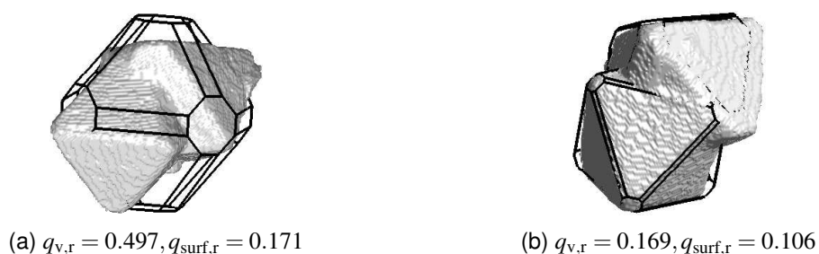
Figure 3.25: Shape identification in case of an aggregate, obtained with the algorithm for single crystals (left) and with the algorithm for aggregates(right). Error measures regarding the right crystals are defined in chapter 4 on crystal aggregates.
