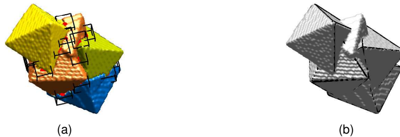
Figure 4.11: Segmentation (left) and shape identification (right) for one aggregate from sample A3-0.2. The orange primary particle was wrongly concatenated with the part of another particle. However, the shape of the orange particle was identified correctly in spite of this segmentation error. The aggregate is considered to contain primary particles where no shape identification was possible by the quality measures developed for simulated data. It is considered to have a successful shape identification by the quality measures for real data.
