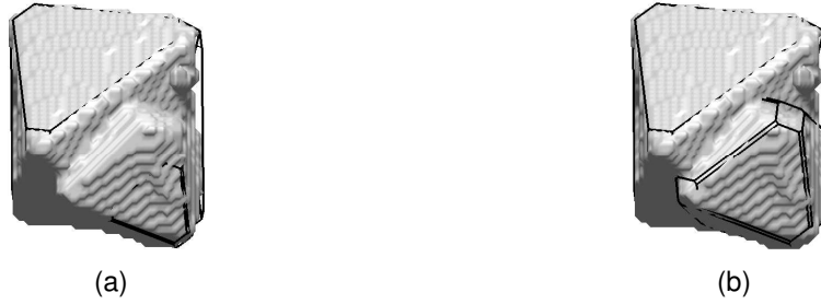
Figure 4.7: Before (a) and after (b) moving and re-sizing the smaller primary particle shape fit.
