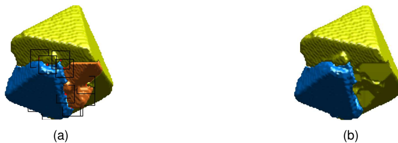
Figure 4.5: Faulty region, presented in orange in the left image is identified and deleted, resulting in the right image. Concavity points are shown in red in the left image.
