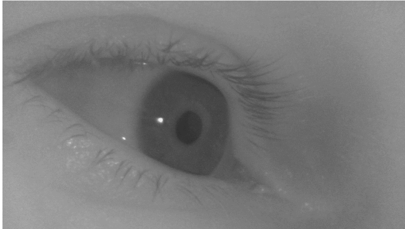
Figure 16: View from the eye tracking headset into the eye. The pupil movement as well as its size in pixel coordinates are extracted from the video stream and used for further calculations.
