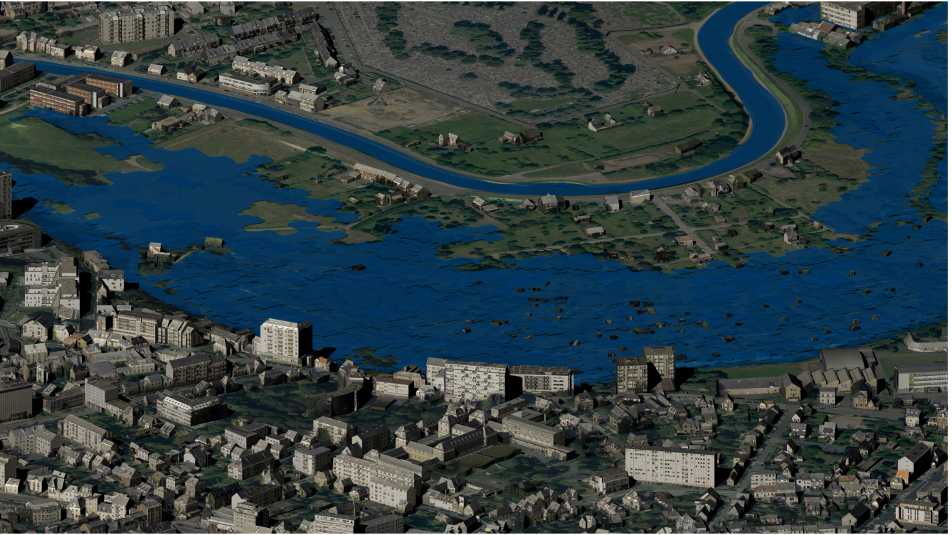
Figure 19. Visualization of flooding in Rennes using the proposed CityGML encoding draped over 3D terrain and building data (provided by Rennes Métropole/IGN).
