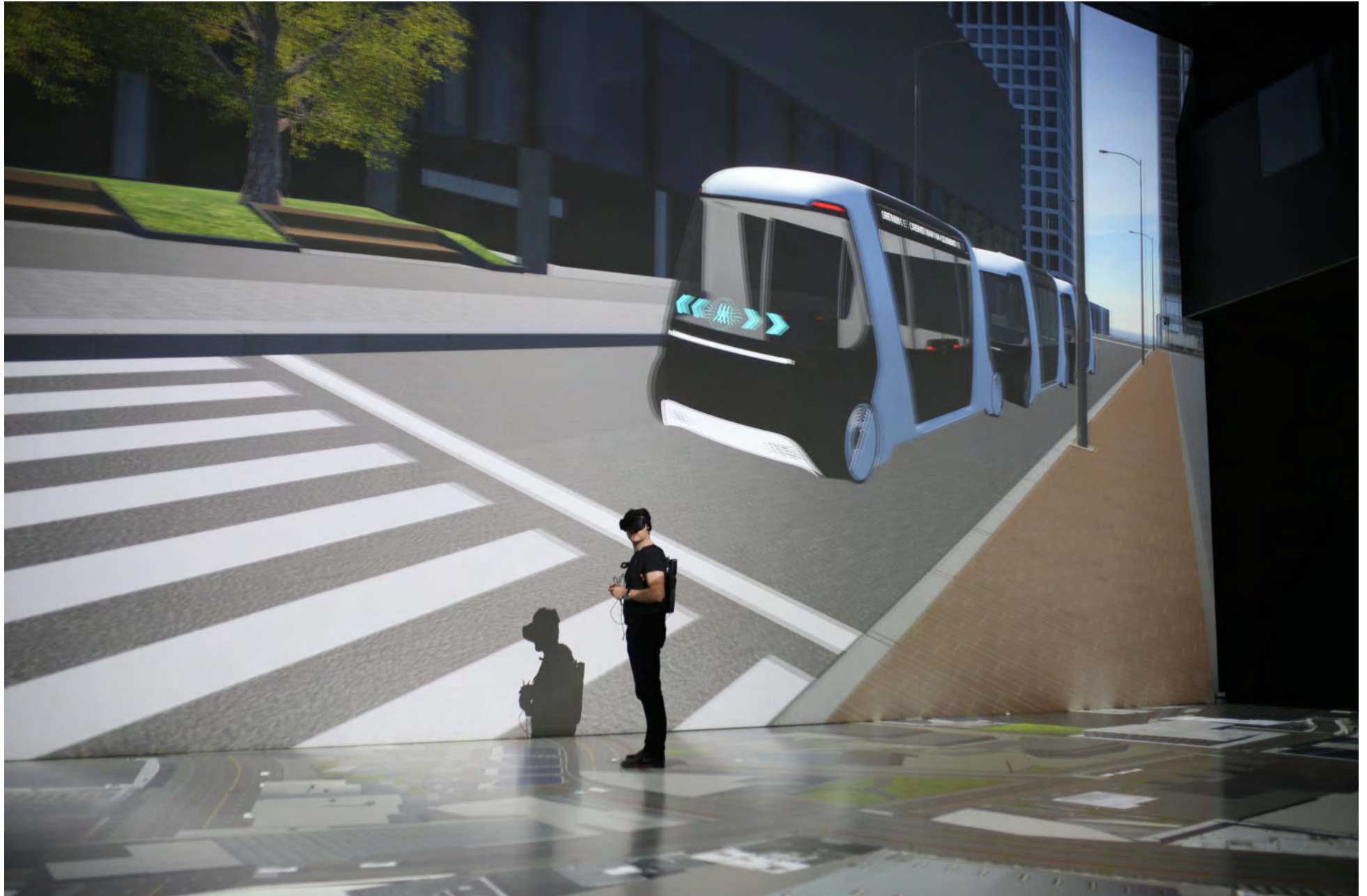
Image 14. Interaction with an AV at a crossing, human in the loop simulation
