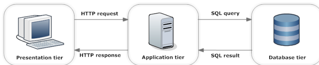
Figure 2.2: Web application architecture. The figure shows three layered architecture of the bioCompendium.
