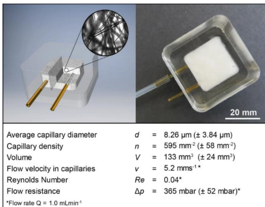
Figure 1: Schematic representation (left) and photograph (right) of the capillary filtration system. Brass tubes serve as in- and outlets into the capillary system, which was generated by leaching out sacrificial sugar structures from the PDMS cube. The production process established here allows for generating filtration devices with reproducible properties as depicted in the table below the pictures.
