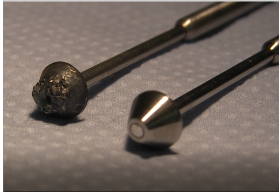
Figure 7.15.: Post-firing view of injector pintle body and replacement.
