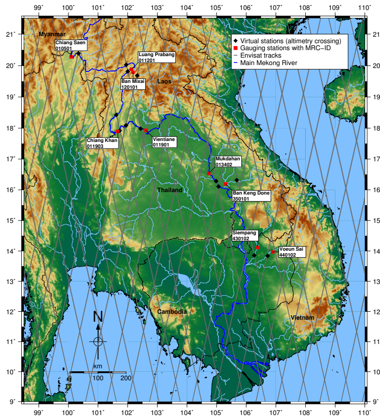
Figure 2. Study area of the lower Mekong River, indicating the gauging stations used in the validation (name of the nearest settlement and ID issued by the Mekong River Commission), the virtual stations, and the Envisat altimetry tracks.
