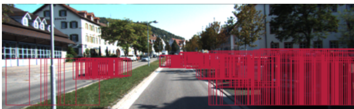
(c) Generated proposals after adjusting the Stixel width.
