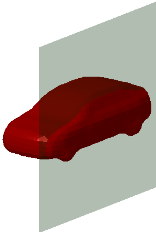
Figure 4.3: Visualization of a three-dimensional SDF.
