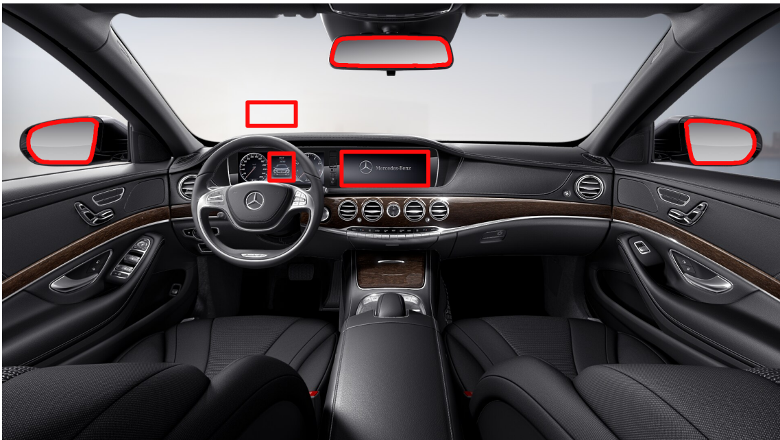
Figure 5.15: Possible display areas in the S-Class AR prototype vehicle. Image source: Daimler AG. Adapted by the author.
