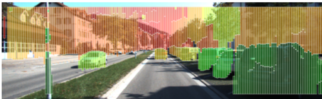
(a) Stixels generated by a stereo camera.
