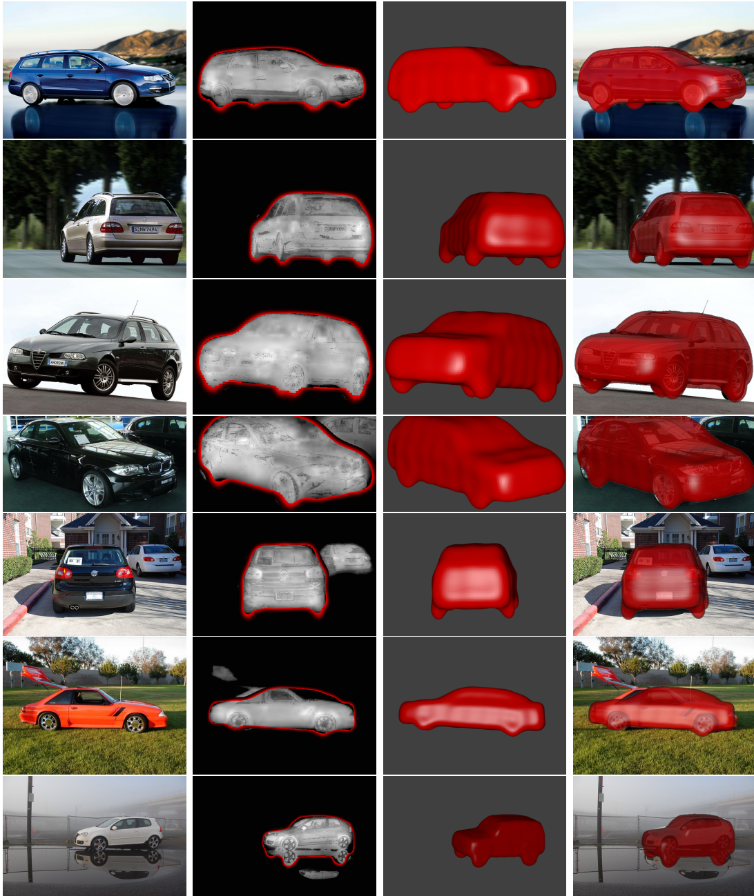
Figure 4.16: More reconstruction results of monocular 3D Shaping. The last two rows present two failed reconstructions due to 180°-flipped viewpoint and strong reflection from the wheel, respectively.
