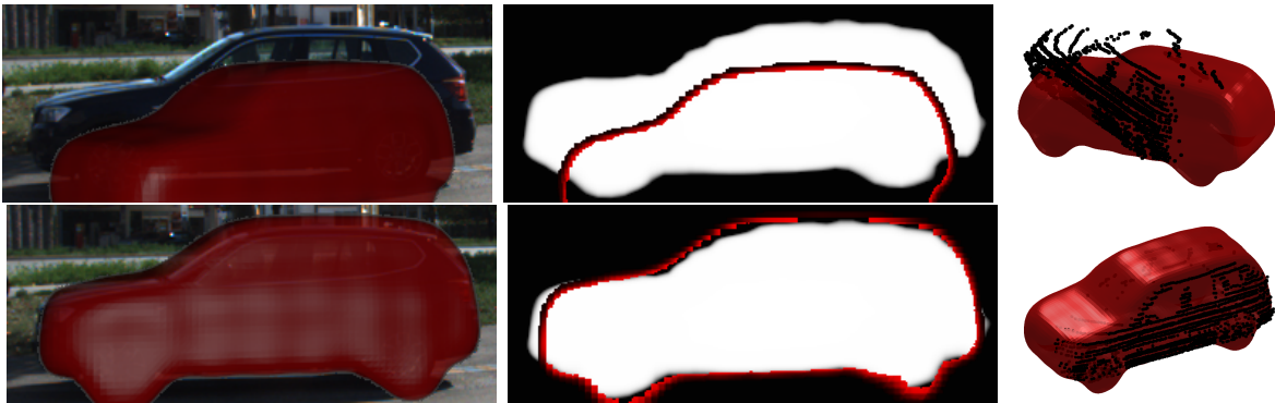
Figure 4.21: 3D Shaping optimization using image and Lidar measurements. The first row shows the initial state, and the second row the final state. Image statistics are illustrated in the middle column, with white pixels being more likely to be foreground pixels. The right column shows SDFs and Lidar measurements.
