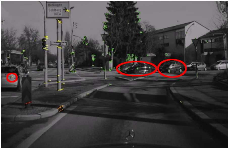
Figure 5.27: Elimination of outliers by ego-motion estimation using semantic information. Feature points inside the red eclipses are identified car pixels and thus excluded from the feature pool.
