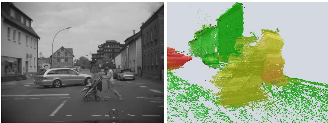
Figure 1.9: Example of 6D Vision. The left image shows a typical traffic scene. The right image draws the dense motion field of the surroundings estimated using 6D Vision. Velocities are encoded in color from green being slow to red being fast. Images are extracted from [RMWF10] and adapted by the author.
