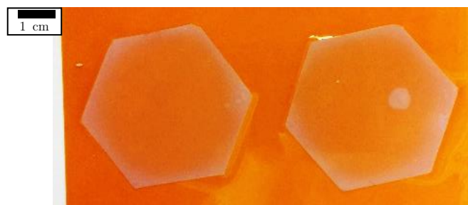
Figure 3.29. Two non-stretchable pieces of coated PET surrounded by elastic PDMS on a Kapton carrier material. The non-stretchable parts could serve as high-resolution inkjet-printing of a complex circuitry that is connected elastically to each other after peeling off from the carrier material.
