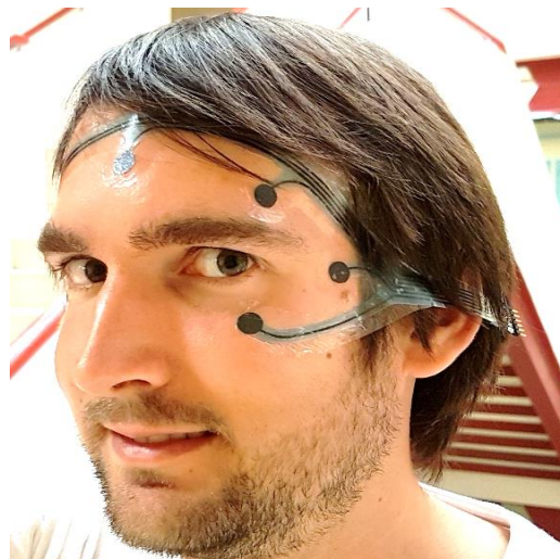
Figure 4.53. EOG skin patch with carbon electrodes attached to the forehead of the author.
