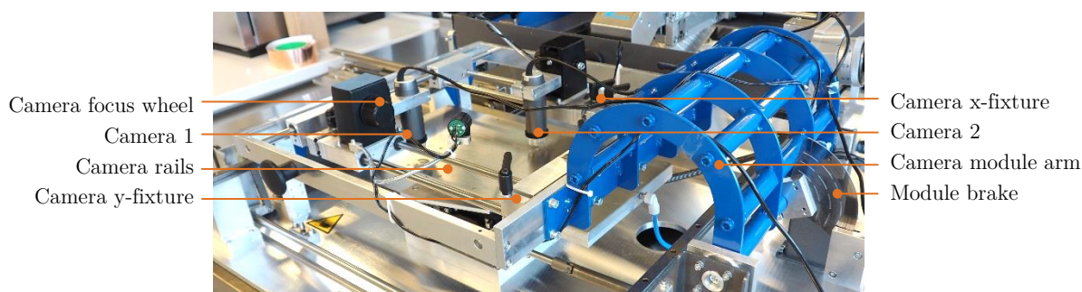
Figure 2.28. The camera module of the screen printer Nino with two cameras that can be precisely moved in two directions and tightly fixed at the desired positions.
