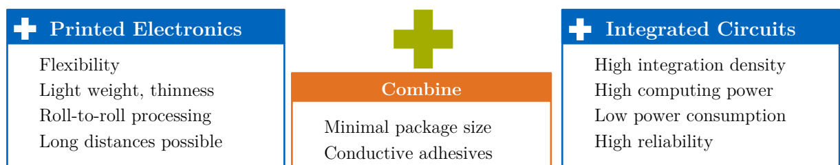
Figure 5.1. Hybrid systems combine the advantages of Printed Electronics and silicon-based Integrated Circuits to create attractive new devices.
