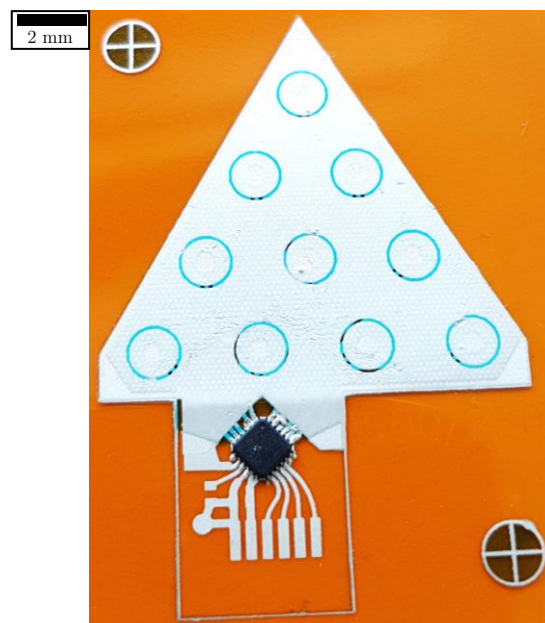
Figure 5.30 Bottom layer of the force sensing triangle with attached CDC.
