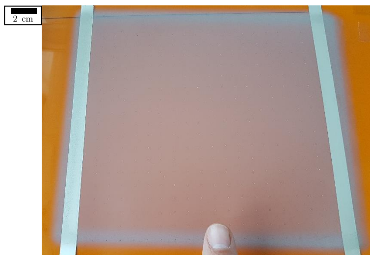
Figure 3.22. Large area transparent heater with screen-printed bar electrodes and spray-AgNWs.
