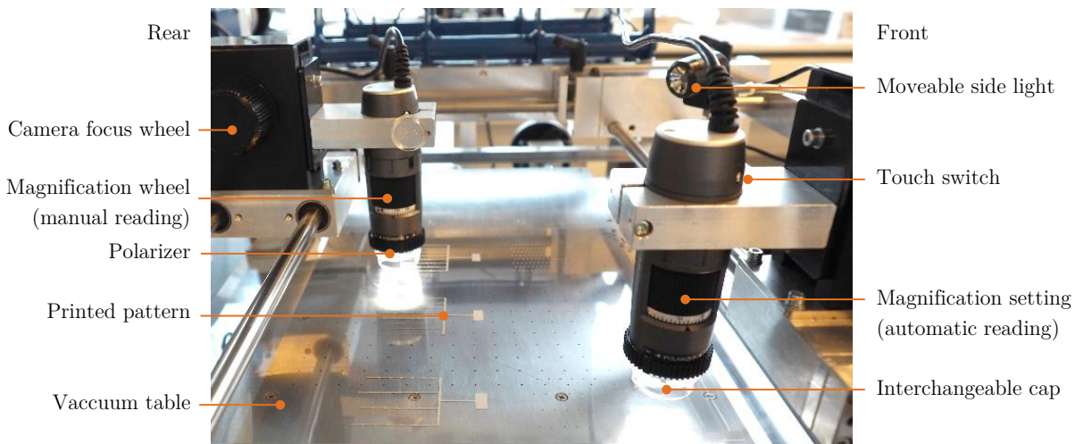
Figure 2.29. Close view on the cameras of the print module in the Nino printer.
