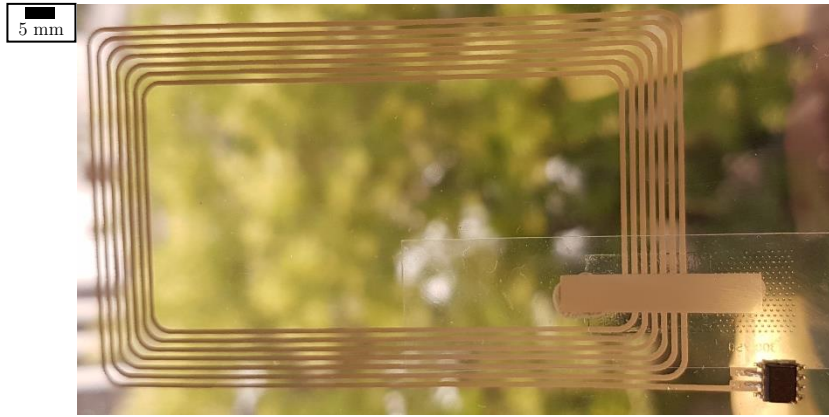
Figure 5.8. Screen-printed NFC antenna with the assembled chip.
