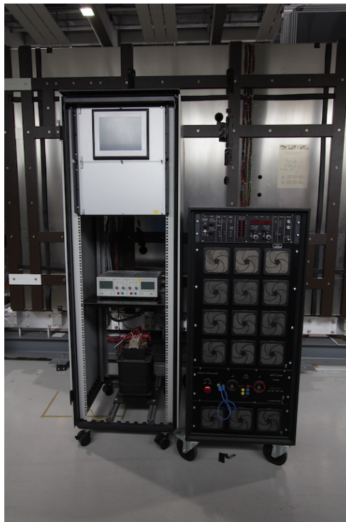
Figure 3.3: Photograph of the equilibration setup. A 19-inch rack houses all of the equipment, except the amplifier. On the top a touch screen PC allows control of the process. The (closed) relay box below the PC distributes the current, after it has been filtered by 80 kg transformer on the bottom. The amplifier comes in its own movable rack.
