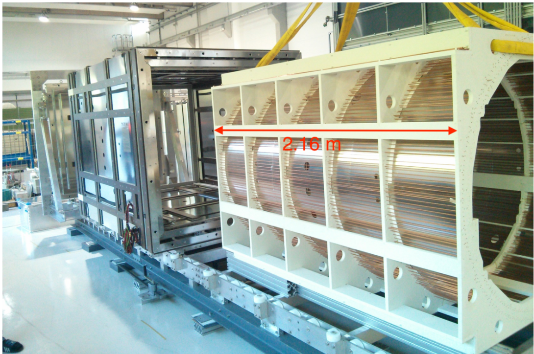
Figure 2.10: Photograph taken during the assembly of the insert and the cylindrical shield with the B_0 coils. The printed circuit boards (PCBs) that connect the individual tubes to form single or multi-turn coils were not yet mounted for this picture.
