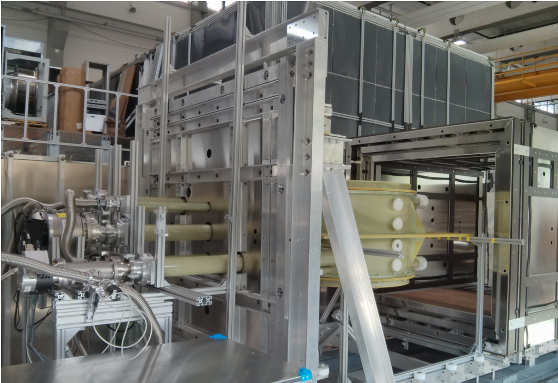
Figure 2.11: Photograph of the test assembly, where the vacuum chamber has been mounted in the back door of the insert and was evacuated.
