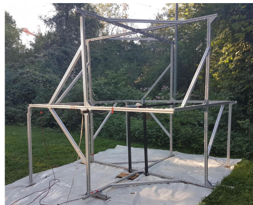
(b) Three square calibration coils.
